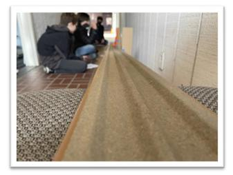
Above: Middle schoolers have recreated Galileo's acceleration demonstration on three different scales (6', 9', and 20'). They recorded times based on the four equal distances. Then Physics students again crunch numbers to prove acceleration happens and divide the ramp into four equal TIME segments.
